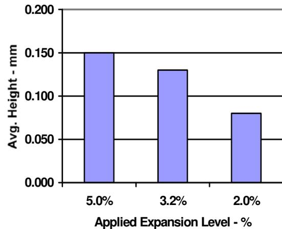
Figure 3 – Height of volcano as a function of applied expansion
