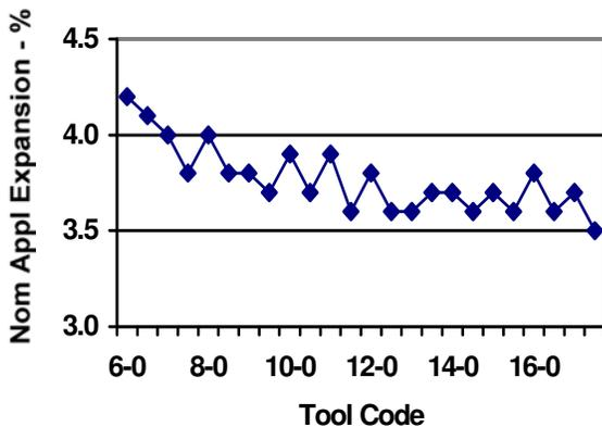
Figure 5 - Nominal Applied Expansion Levels for Split Sleeve Process.
