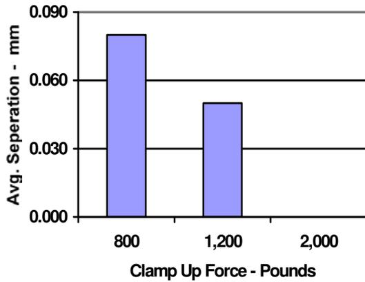
Figure 4 - Stackup separation vs. clampup forces
